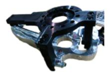
All Greening test fixtures are surface coated with **black oxide** to inhibit corrosion.
